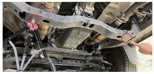
3.) Identify the two holes shown in the picture on the transmission crossmember - these are located just to the inside (and forward) of the holes from the previous step. Drill them out with a 25/64" drill bit, then install the SHORT  $\frac{1}{4}$ " rivnuts into the 2 holes.
