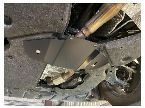
11.) Install your main catalytic converter piece using the 5/16"- $18 \times 1$ " long bolts with blue thread locker on the threads. Securely tighten these 5 bolts. Don't over tighten or you will strip the bolt heads.
