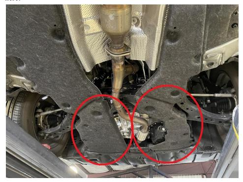
3.) Remove the 8 clips circled that hold the covers - use a flat head screwdriver.
