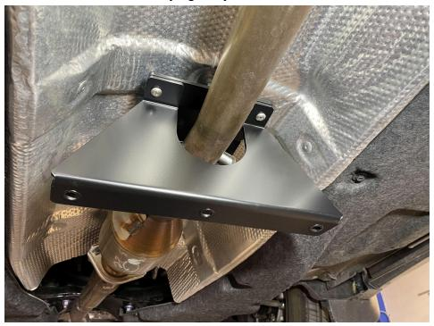
10.) Install your front bracket now. The front bracket is mounted to the rivnuts you installed earlier. Use the  $\frac{1}{4}$ "-20 x 2.75" security bolts with the  $\frac{1}{4}$ "x1" washers under the bolts heads; put threadlocker on the bolt threads. The 35mm spacers fit between the bracket and vehicle where the bolts push up. Use the 5/32" security bit. Leave loose.
