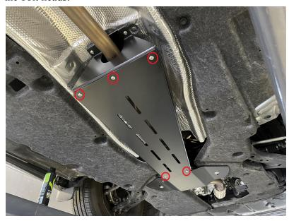
12.) Tighten the 2 bolts on the front bracket and the 2 bolts on the rear bracket. Allow the threadlocker to cure for at least 15 minutes before driving.
