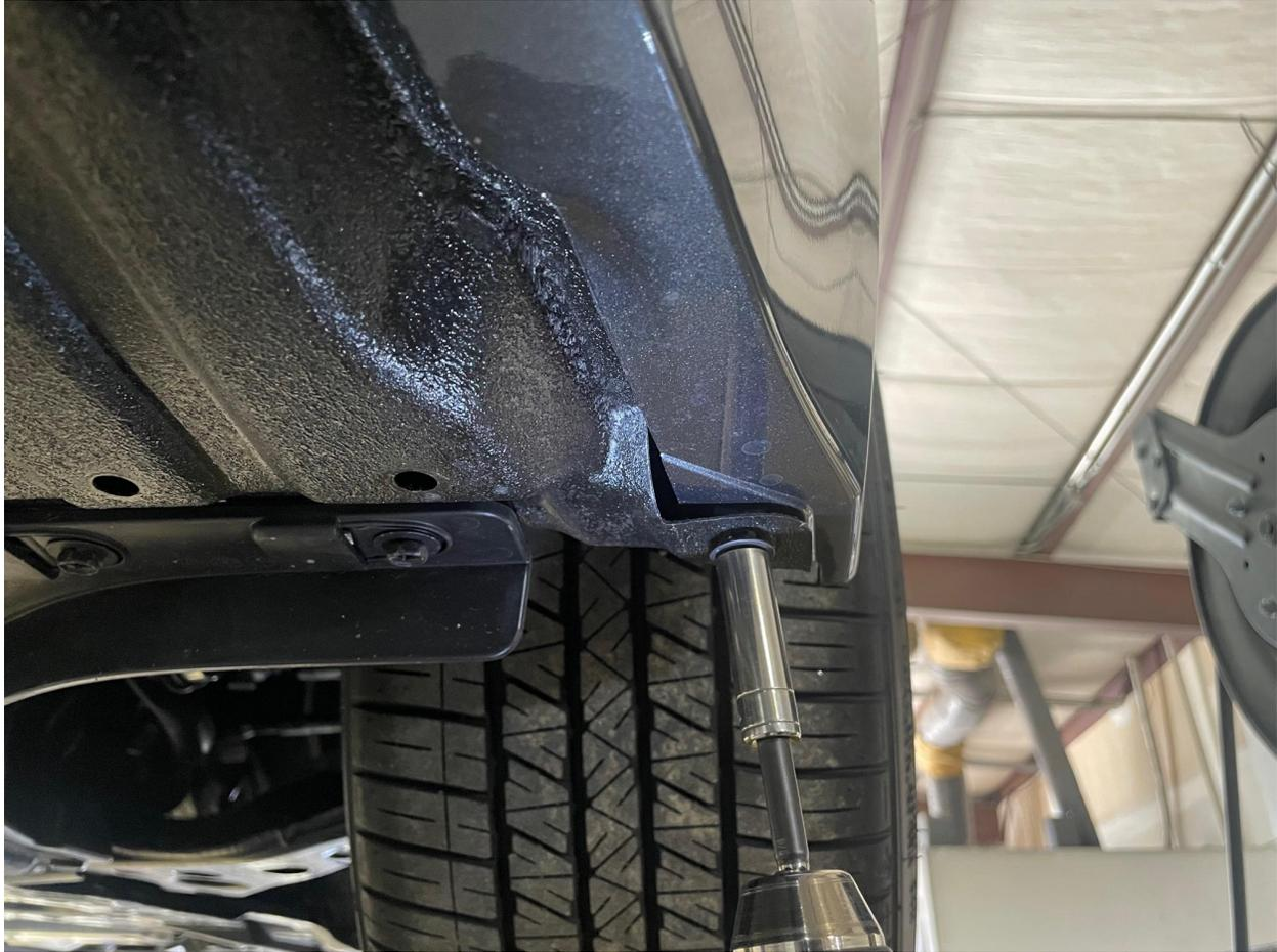
4.) Install your splitter onto the vehicle using the screws just removed. Don't overtighten; the screws will simply just keep spinning if you do.
