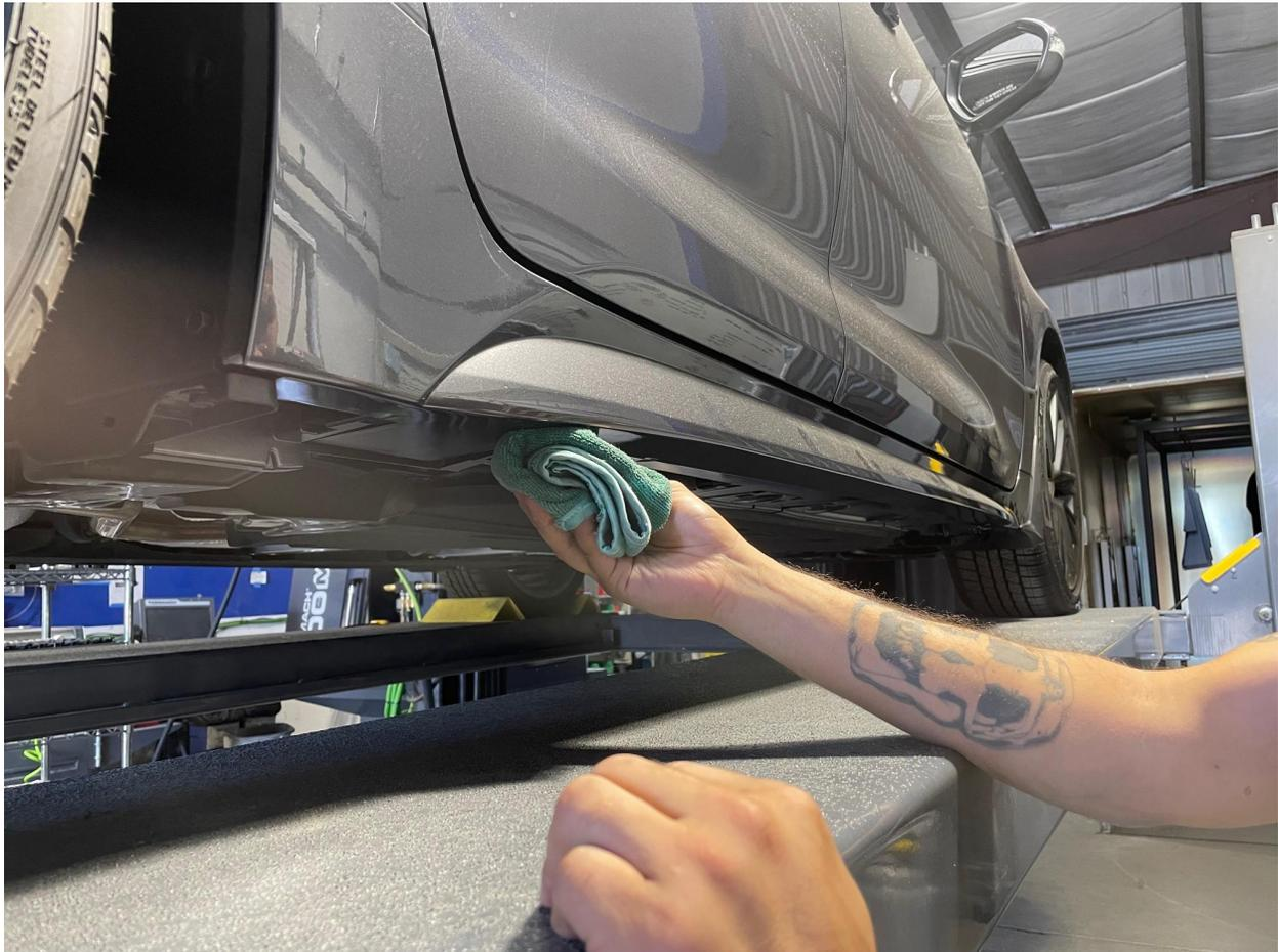
3.) Hold the side skirt up against the underside of the rocker panel. The inside of the side skirt extension should follow the straight inner edges of the pockets in the rocker panel. Figure out the best position where the tape will stick the entire length.
