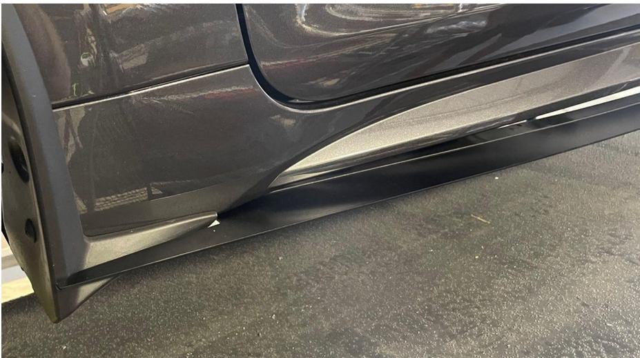
4.) This step is optional. If you'd like to secure the side skirt additionally, you can install the supplied screws. These screws are mounted through the holes located at the front and rear of the side skirt, and up into the rocker panel. We recommend drilling a 5/64" hole at those locations if you're going to do so.
