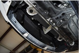
8.) Install your splitter into the holes along the bumper - the 2 OEM spots on the left and right edges, and the 4 drilled holes. Use M6-1.0 x 70mm bolts with 1" OD fender washers on top and bottom and M6 nyloc nuts on top (nuts only for the 4 drilled holes) - **USE 50MM SPACERS BETWEEN THE SPLITTER AND BUMPER IF YOU HAVE A LIP**. Securely tighten.
