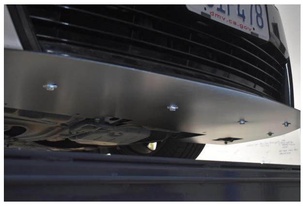
10.) We are on the home stretch. There are 5 holes left in the splitter at the rear. The holes at the most outer left & outer right use M6-1.0 x 130mm bolts and 114mm spacers. The inner three use M6-1.0 x 120mm bolts and 103mm spacers. Use  $\frac{1}{4}$ " lock washers and 1" OD fender washers under the heads of the bolts, and place the spacers between the splitter and car. The bolts will thread into the existing holes in the car.
