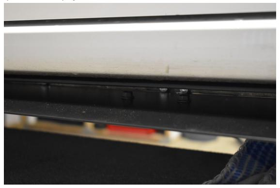
12.) Lastly, there is a hole at the rear of the skirt. You need to drill up through it with a  $\frac{1}{4}$ " drill bit and make a hole in the car.
