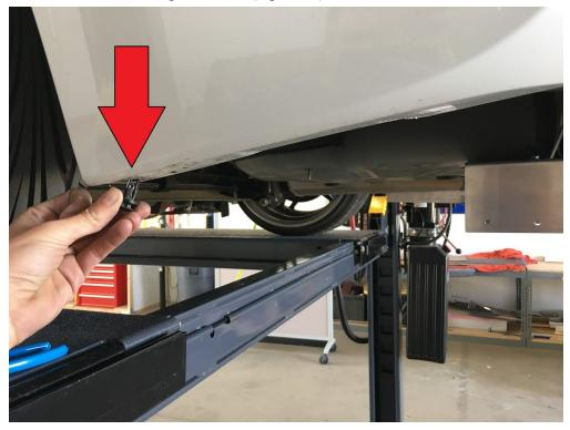
6.) Install your outer pieces onto the center diffuser. Use M6-1.0x12mm bolts and M6 nyloc nuts. The bolts can be pointed upward or downward. (2 pictures)
