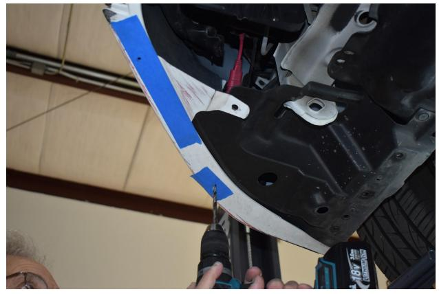
6.) Next, swap to a 5/16" drill bit. We are now going to drill through your crash bar. Locate the 3 holes in the following picture. Push your drill bit through the bottom holes up until it touches the top portion of the crash bar. Drill a hole in the top portion. TAKE YOUR TIME.
