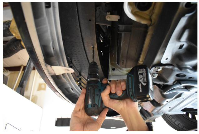
7.) Install your 3 round crash bar mounts. Push the thread through the bottom and newly drilled top holes in the crash bar. Use a 5/16" ID small washer and 5/16"-18 nyloc nut on the top. To tighten use a  $\frac{1}{2}$ " wrench to turn the nut while gripping the crash bar mount.
