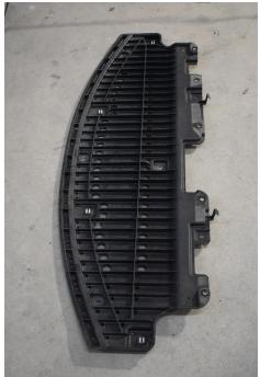
3.) We want to "square up" the splitter. First remove and discard the "flaps" on either side of the bumper underside. Locate the 10mm screws at the left and right edges of the bumper. Install your splitter into those two holes. The back edge of the splitter should sit against the front edge of the inner fender well. Make sure the same amount of splitter is sticking out on the left and right sides of the bumper.
