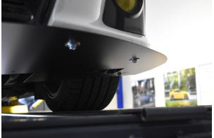
9.) Next install your 5/16"- $18 \times 3/4$ " long bolts into the crash bar mounts. If you did not drill perfectly vertically, you will need to reach in behind the splitter and move the mounts so they line up. This is where a friend and a lift come in handy. Use 5/16" ID, 1" OD fender washers under the heads and blue threadlocker on the bolts.
