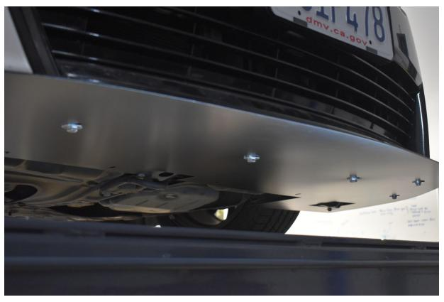
10.) We are on the home stretch. There are 5 holes left in the splitter at the rear. The holes at the most left and right use M6-1.0 x 80mm bolts and 64mm spacers. The inner three use M6-1.0 x 70mm bolts and 53mm spacers. Use  $\frac{1}{4}$ " lock washers and 1" OD fender washers under the heads of the bolts, and place the spacers between the splitter and car. The bolts will thread into the existing holes in the car.
