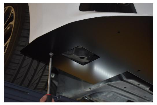
4.) If your corolla is a dark color, place tape on the underside of the bumper where the 4 holes are located in the splitter along the perimeter of the bumper. If it's a light color don't worry about the tape. Use your sharpie/marker to mark through those four holes onto the bumper. Then remove the splitter.
