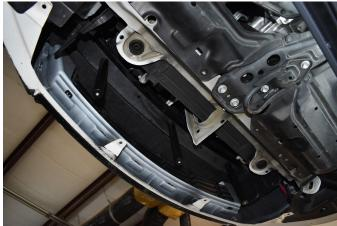
8.) Install your splitter into the holes along the bumper - the 2 OEM spots on the left and right edges, and the 4 drilled holes. Use M6-1.0 x 20mm bolts with 1" OD fender washers on top and bottom, and M6 nyloc nuts on top. Securely tighten.
