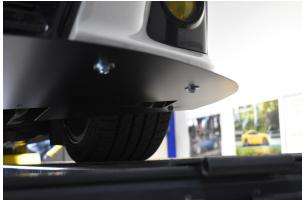
9.) Next install your 5/16"- $18 \times 3/4$ " long bolts into the crash bar mounts. If you did not drill perfectly vertically, you will need to reach in behind the splitter and move the mounts so they line up. This is where a friend and a lift come in handy. Use 5/16" ID, 1" OD fender washers under the heads and blue threadlocker on the bolts.
