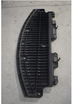
3.) We want to "square up" the splitter. Locate the 10mm screws at the left and right edges of the bumper. Install your splitter into those two holes. The back edge of the splitter should sit against the front edge of the inner fender well. Make sure the same amount of splitter is sticking out on the left and right sides of the bumper.
