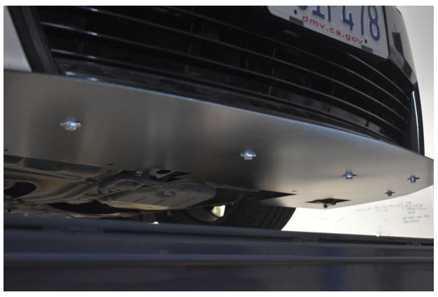
10.) We are on the home stretch. There are 5 holes left in the splitter at the rear. The holes at the most outer left & outer right use M6-1.0 x 120mm bolts and 99mm spacers. The inner three use M6-1.0 x 110mm bolts and 88mm spacers. Use  $\frac{1}{4}$ " lock washers and 1" OD fender washers under the heads of the bolts, and place the spacers between the splitter and car. The bolts will thread into the existing holes in the car. Securely tighten.
