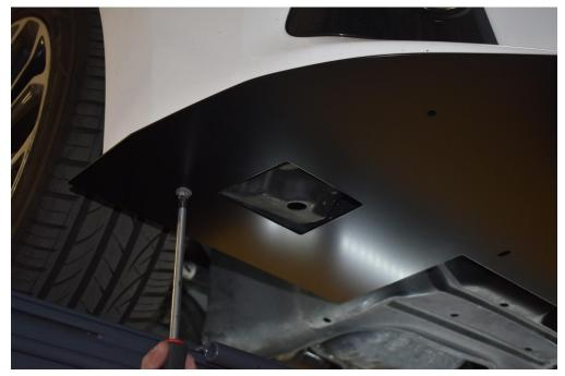
4.) If your corolla is a dark color, place tape on the underside of the bumper/lip where the 4 holes are located in the splitter along the perimeter of the bumper/lip. If it's a light color don't worry about the tape. Use your sharpie/marker/pencil to mark through those four holes onto the bumper/lip. Then remove the splitter.
