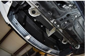
8.) Install your splitter into the holes along the bumper - the 2 OEM spots on the left and right edges, and the 4 drilled holes. Use M6-1.0 x 65mm bolts with 1" OD fender washers on top and bottom and M6 nyloc nuts on top (nuts only for the 4 drilled holes) - USE 45MM SPACERS BETWEEN THE SPLITTER AND BUMPER IF YOU HAVE A LIP. Securely tighten.
