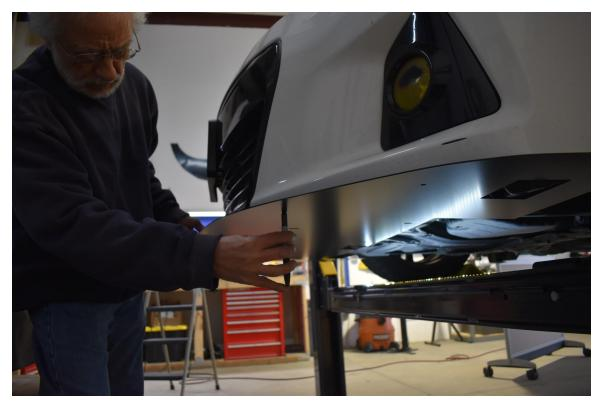
5.) Assure the splitter is spaced from the bumper equally on the left and right. Grab your drill. Drill ¼" holes through the bumper into the spots you just marked from the previous step. If you have a lip you will likely be drilling through it as well. Then remove the tape if any was used.
