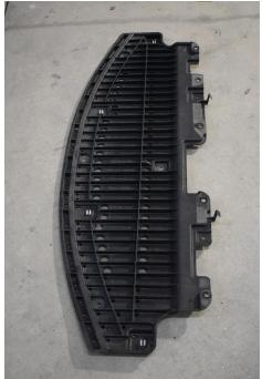
3.) IF YOU HAVE A THREE PIECE SPLITTER we recommend bolting the splitter together temporarily for steps 3-5. Use the common bolt holes among the pieces. Use four M6-1.0 x 20mm bolts and whiznuts.
