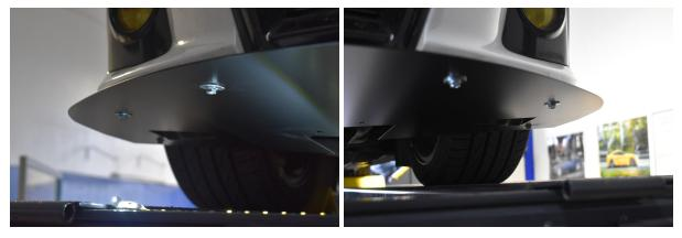
9.) Next install your 5/16"- $18 \times 3/4$ " long bolts into the crash bar mounts. If you did not drill perfectly vertical, you will need to reach in behind the splitter and move the mounts so they line up. This is where a friend and a lift come in handy. Use 5/16" ID, 1" OD fender washers under the heads and blue threadlocker on the bolts.
