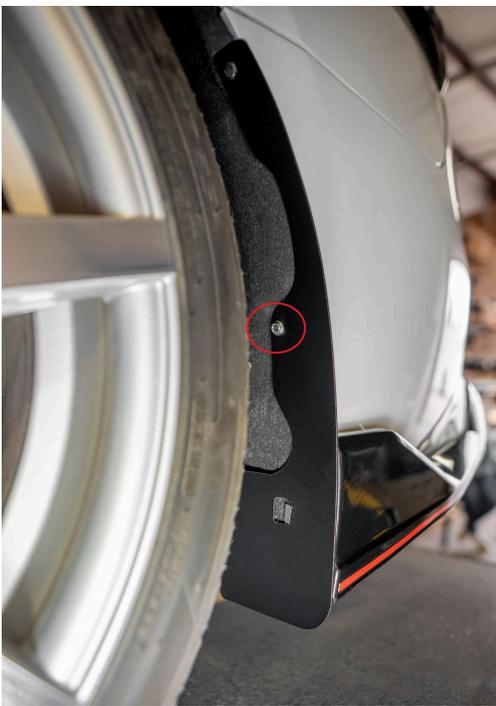
Make sure you're pushing the guard up against the car when tightening the bolt. Stop when it feels very snug and cannot be pulled back out. Get help from a friend here!
