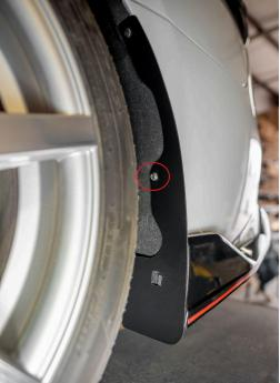
Make sure you're pushing the guard up against the car when tightening the bolt. Stop when it feels very snug and cannot be pulled back out. Get help from a friend here!
