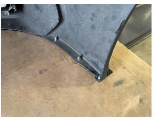
5.) DOUBLE CHECKING CENTER AND MARKING FOR OTHER HOLES \ REMOVED CENTER PIECE, DRILLED INNER TWO HOLES, REINSTALLED CENTER WITH NYLOC NUTS.
