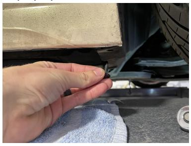
3.) In front of the rear wheel is an empty hole (at least ours was empty). It looks like a clip may have slid inside of it possibly to hold up the rear "flap" that hangs down. Remove whatever is blocking the hole and drill it out to a ½" hole. This will be the rear most mounting point for the skirt. Here is the location of the hole.
