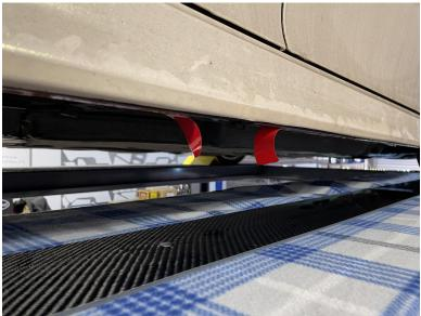
8.) Side skirt installation can now be done. Use the well nuts with associated bolts for the rear and center hole, and OEM screw for the front. Leave them loose and peel the 3M backing off. Firmly press upward and hold each part of the side skirt against the rocker panel for at least 20 seconds to assure the 3M tape does the job. Then tighten the well nuts and screw.
