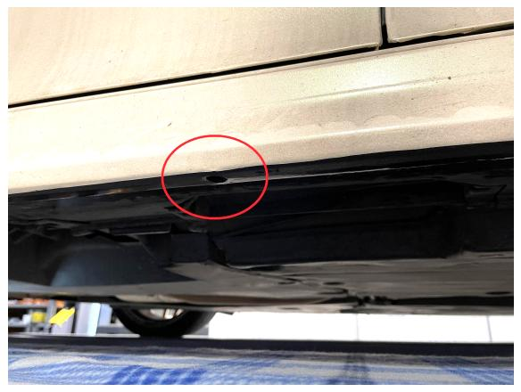
6.) Now it's time to thoroughly clean the underside of the OEM rocker panel using your cleaning supplies, and isopropyl alcohol. Clean it until there is no more dirt. Then you need to apply 3M tape onto the OEM rocker panel between the side skirt mounting holes. Make sure the tape is continuous between the holes. Firmly press to assure the 3M tape sticks.
