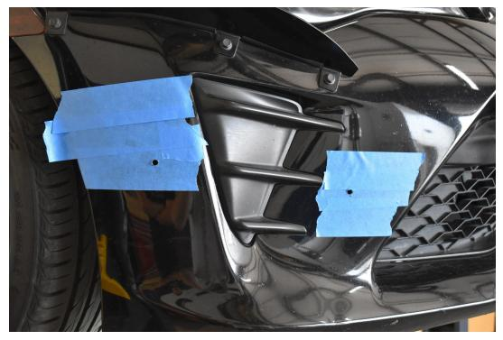
6. Install the canard with both wiznuts Remove the canard and reinstall it with the countersunk bolts/washers & ¼" small washers/nyloc nuts on the inside. Use the rubber washers between the tabs on the canard and bumper. (2 PICS)
