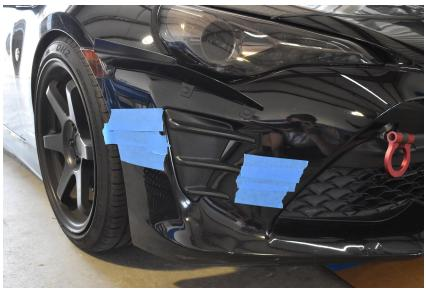
3. With help from a friend hold the canard up against the car so it contours the middle fin as best as possible. Mark the hole toward the front of the car with a pen. Then make a hole at that spot with your drill and ½" drill bit. (2 PICS)
