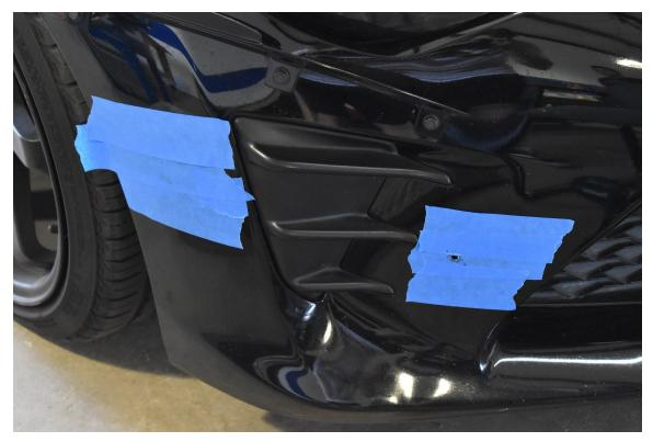
4. Underneath the front bumper remove the 10mm head bolt that helps holds the outer undertray on. This will gain you access to behind the bumper. (1 PIC)
