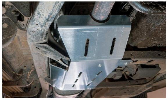
6.) Securely tighten all 4 bolts. You will need to hold the nuts on top. The  $\frac{1}{4}$ " bolts use a  $\frac{7}{16}$ " wrench, and the  $\frac{5}{16}$ " bolts use a  $\frac{1}{2}$ " wrench.
