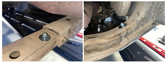
4.) Then loosely mount the guard onto the vehicle at the front 2 points. View from the top looks about the same as the 2 shown above, just in different locations.
