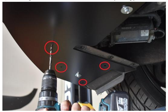
6.) Drill through the outer 4 holes on each side of the bumper using your  $\frac{1}{4}$  drill bit.
