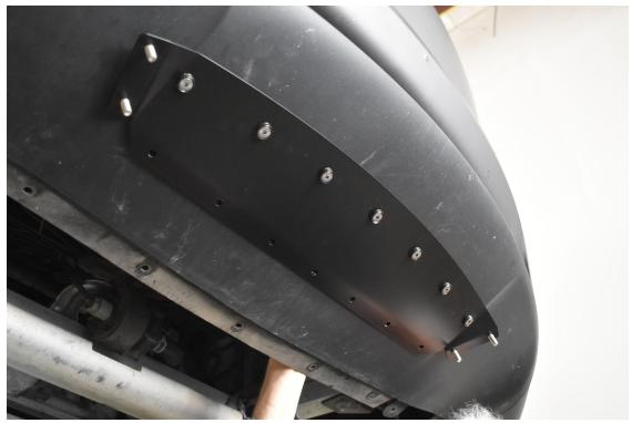
9.) Now it is time to install your splitter onto your reinforcing bracket. Use the  $\frac{1}{4}$ " small washers and  $\frac{1}{4}$ "-20 nyloc nuts on the hex head bolts underneath the splitter. Securely tighten. You will need to use the 7/16" wrench on the top of the splitter and the 7/16" on the bottom for the nuts.
