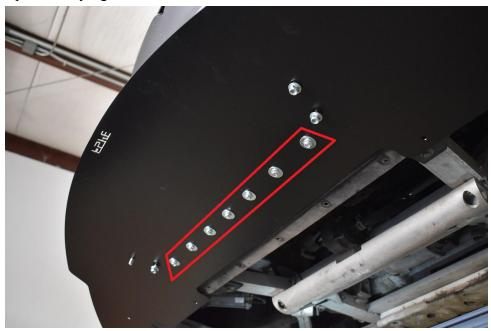
11.) Install your bottom layer splitter pieces onto the top layer splitter on the left and right sides. (one side shown). These pieces are symmetrical. Leave the OEM hole on each side open. Use M6-1.0 x 20mm bolts with  $\frac{1}{4}$  x 1" washers on bottom & top, and M6 nyloc nuts on top. Securely tighten.
