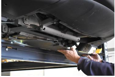
4.) Your splitter is in pieces. The top layer is the largest piece of the splitter. Install your top layer onto the 4 locations shown in the following pictures.
