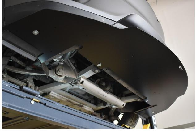
5.) Locate the back row of holes at the center on the top layer splitter. You need to drill  $\frac{1}{4}$ " holes through the splitter holes into the plastic bumper. There are 7 holes.
