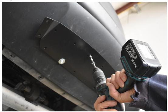
8.) Once the 7 holes are drilled push the  $\frac{1}{4}$ "-20 x 0.75" hex head bolts downward through the outer holes in the reinforcing bracket (first pic).
