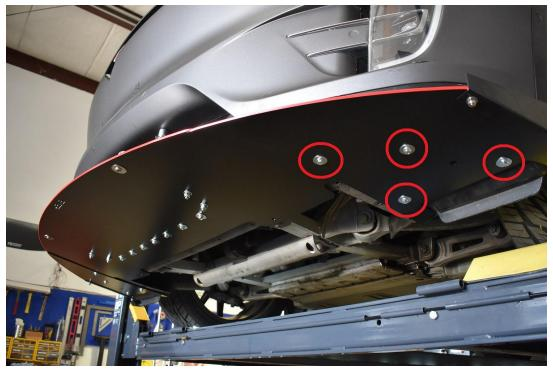
12.) Install your flares. There is a left and right side. Use the remaining countersunk stainless steel bolts ( $\frac{3}{4}$ " long) with the associated countersunk washer, and  $\frac{1}{4}$ " small washer +  $\frac{1}{4}$ "-20 nyloc nut. Securely tighten.
