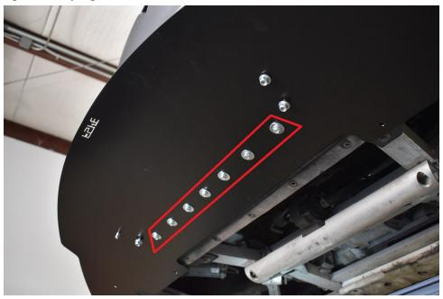
11.) Install your bottom layer splitter pieces onto the top layer splitter on the left and right sides. (one side shown). These pieces are symmetrical. Leave the OEM hole on each side open. Use M6-1.0 x 20mm bolts with 1" washers on bottom & top, and M6 nyloc nuts on top. Securely tighten.
