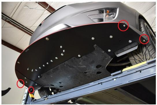
13.) Reinstall your under tray using the OEM clips and bolts. Except, replace the front two bolts with M6-1.0 x 30mm long bolts. Use  $\frac{1}{4}$ " lock washers and 1" OD washers under the heads. Securely tighten.
