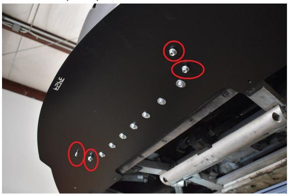
10.) Install M6-1.0 x 20mm bolts into the 7 holes that are common in both the reinforcing bracket and top layer splitter. Use 1" washers on bottom, and  $\frac{1}{4}$ " washers + M6 nyloc nuts on top. Securely tighten.
