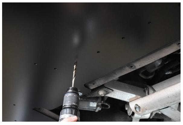
6.) Drill through the outer 4 holes on each side of the bumper using your 1/4" drill bit.
