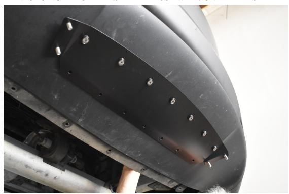
9.) Now it is time to install your splitter onto your reinforcing bracket. Use the stainless steel  $\frac{1}{4}$ " washers and  $\frac{1}{4}$ "-20 nyloc nuts on the hex head bolts. Securely tighten. You will need to use the  $\frac{1}{2}$ " wrench on the top of the splitter and the  $\frac{7}{16}$ " on the bottom for the nuts.
