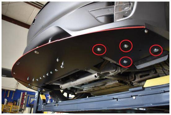
12.) Install your flares. There is a left and right side. Use the remaining countersunk stainless steel bolts ( $\frac{3}{4}$ " long) with the associated countersunk washer, and  $\frac{1}{4}$ " SS washer +  $\frac{1}{4}$ "-20 nyloc nut. Securely tighten.
