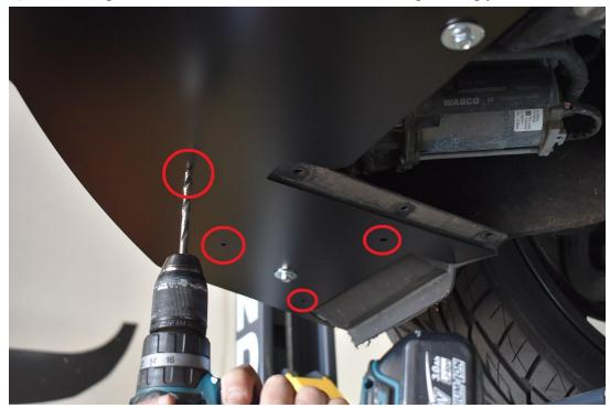
7.) Remove your top layer splitter and temporarily install your reinforcing bracket using two M6-1.0 x 20mm long bolts with 1" washers on top/bottom and whiznuts. The upward angle of the bracket matches the upward angle of the bumper. Drill through the front row of holes (there are 7).
