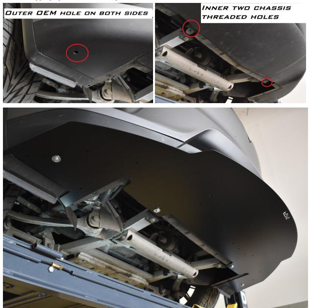
5.) Locate the back row of holes at the center on the top layer splitter. You need to drill ¼" holes through the splitter holes into the plastic bumper. There are 7 holes.
