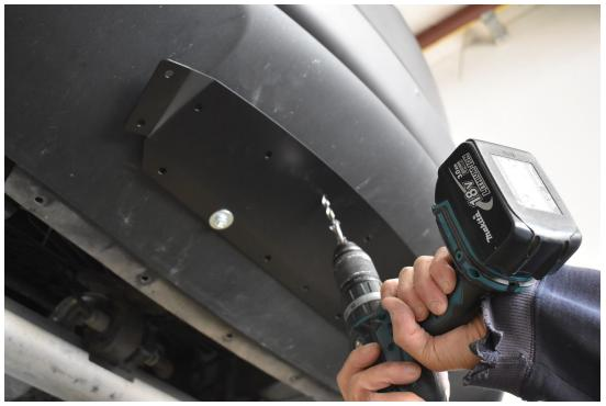
8.) Once the 7 holes are drilled install the ¼" hex head bolts downward through the outer holes in the reinforcing bracket. Then install your ¼" countersunk hardware through the reinforcing bracket and bumper. Use the ¼" washers and nyloc nuts on top. Use WD-40 or oil on the bolt threads before tightening the nuts. Securely tighten.
