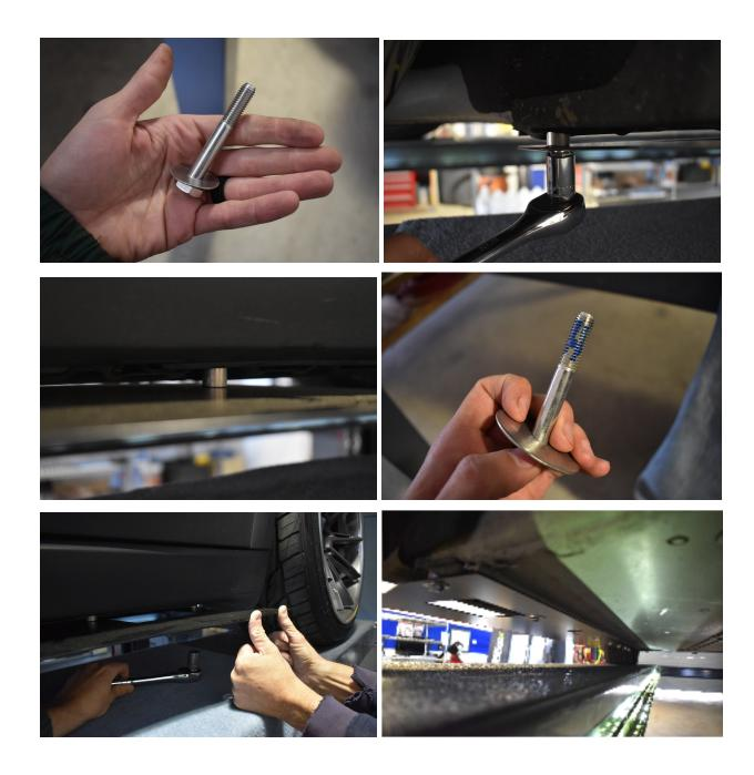
6.) Once all bolts are securely tightened. Install the fins. They each can only go on one side. Use the countersunk bolts and washers, and the ½" small washers and nyloc nuts. The second bracing piece uses the common bolt hole under the fin.
