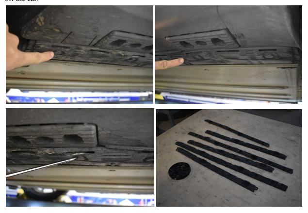
4.) Once the trim is off you'll find several holes above it. Inside 8 of the holes on each side there are bolts with 13mm heads. Remove all 16 of them. They are held with loctite so put some muscle into it! Check out the pictures.
