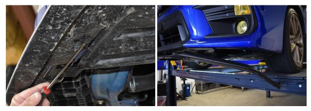
5. Reach your hand through the top of the small plastic tray (it may require moving plastic out of the way) and place a 55mm long bolt + small washer on top facing downward through the hole toward the back of the bumper. Install your driver's side spat loosely with a 30mm spacer, fender washer, and wiznut. (2 pics)
