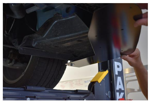
6. Do the same thing for the next hole toward the inside of the spat this using a 33mm spacer and 65mm bolt with a small washer on top and fender washer on bottom. Feel free to point the bolt upward if you'd like but remember to place a small washer inside of the bumper.
