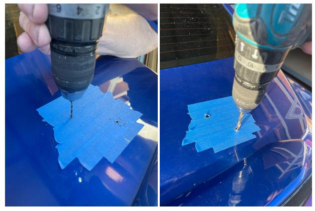
7.) Once the holes have been drilled, assure they are clean and don't have metal protruding around them. Install the wing stands hand tight with the supplied bolts pointing downward into the trunk and whiz nuts on the inside of the trunk. Be very careful when installing the rearward hole as it is easy to drop your whiz nut inside of the trunk. Inner trunk right side shown:
