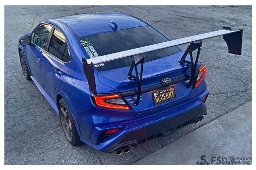
10.) If you haven't already, install your end plates with the smaller bolts using a  $\frac{1}{8}$ " allen key. CFD plates may not be symmetrical, folds go outward. Flat end plates are symmetrical.
