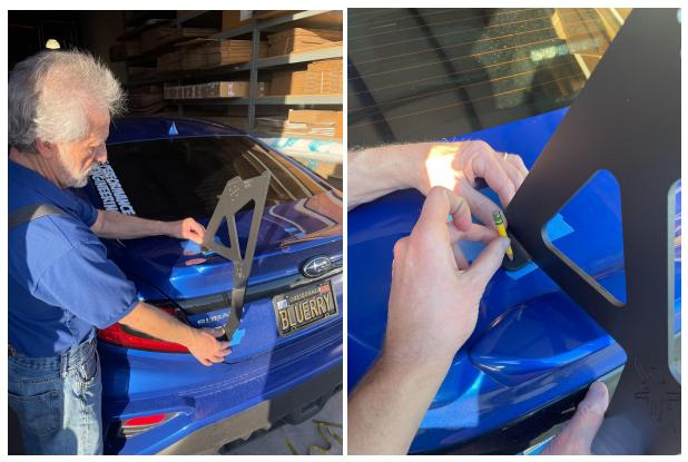
6.) Drill out the top two holes. First use a ½" drill bit to perfectly center the holes, then use a ½" drill bit to open them up. The forward holes on top of the trunk will be passing through two layers of metal when drilling.
