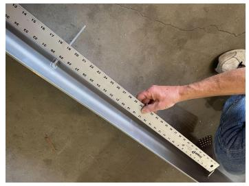
3.) Find the center of your trunk using your measuring tape. Place masking tape onto the trunk and mark the center. Then measure outwards half the distance measured in the previous step (14  $\frac{1}{2}$ "). Place masking tape in that approximate area on each side, then measure exactly  $14 \frac{1}{2}$ " outward from the center to the left and right, make your marks. Double check that the distance between your marks is 29".
