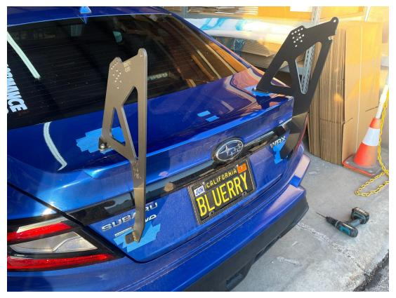
8.) Bolt your wing onto the stands with 2 nuts and bolts on each side.
