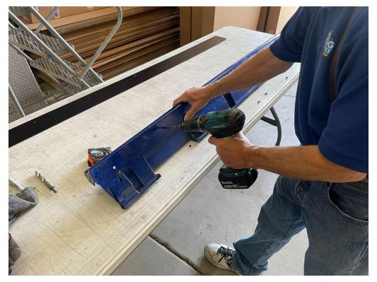
7.) Install your side skirt onto the rocker panel securely (no need to overtighten). Use help from a friend to hold the other end up.
