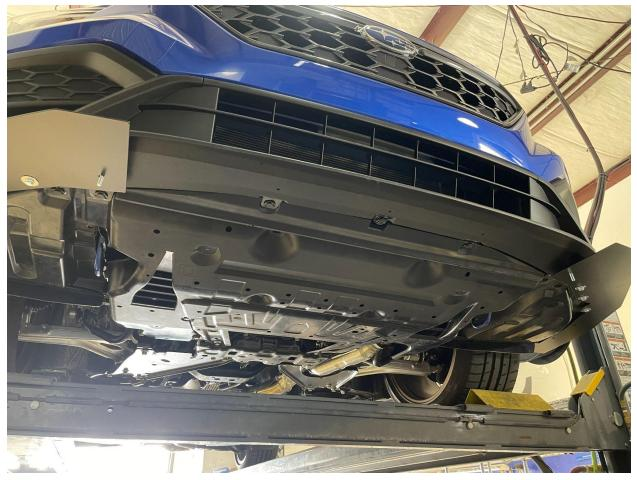
15.) Install your chassis bracket LOOSELY onto the vehicle into the two rivnuts installed, and 12mm bolt locations at the center that hold the center skid plate.
