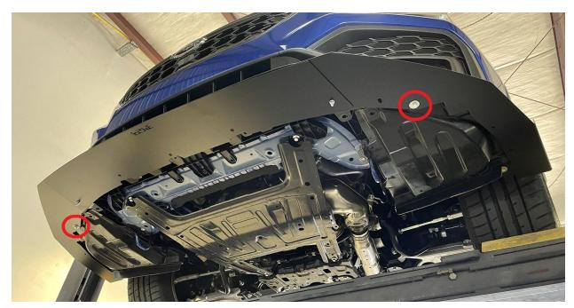
9.) Securely tighten the bolts from step 6. Assure the bolt is indeed passing through the bumper cover/holes and outer skid plate. You'll have to reach above the outer skid plate - try to tighten it so the outer skid plate is about where it needs to be when it's fully installed on the vehicle.
