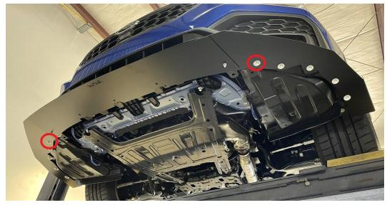
13.) Identify and drill out the hole shown (on each side of the car) with a 17/32" drill bit. Install the supplied 5/16 Rivnuts into the holes shown. Two extra rivnuts are supplied just in case. If you need help understanding a rivnut tool, see the QR code at the beginning of these instructions. **RED ARROW POINTS TO RIVNUT LOCATION (1 on each side of car)**
