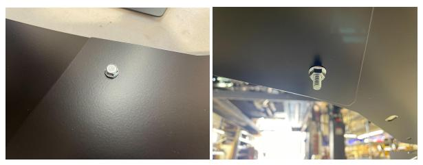
6.) Bolt your splitter onto the car at the most outer holes. Use the M6-1.0 x 30mm bolts, with a  $\frac{1}{4}$ " washer on top and bottom, and nyloc nut on top. These bolts must pass through the bumper cover and outer skid plate. Leave loose. (it will be a far reach on the inside)
