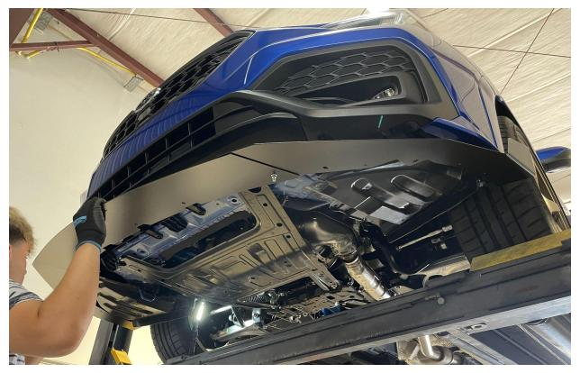
7.) Identify the dimple shown in the bumper cover on each side. These will be located above the splitter. Rotate the splitter out the way, and drill a  $\frac{1}{4}$ " hole through the 2 dimples.
