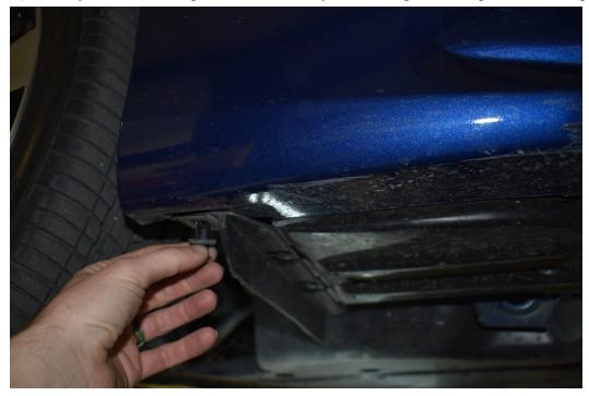
6.) Remove the entire undertray using your flat head screwdriver and phillips head screwdriver. It will make your life MUCH easier. There should be 15 clips (use flat head) and 4 bolts (use phillips head). You'll find them around the front bumper, at the center of the tray, up the sides near the tires, and at the rear of the tray.
