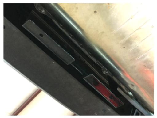
4. Remove the two bolts found on the heat shield on the front side of the rear muffler and install the front bracket at this location. Sandwich it between the heat shield and car. You will need your long extension. Tighten securely. (2 PICS)
