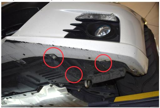
3. Apply painter's tape to the bumper where the canard will mount. Push the canard against the car to locate these spots. (1 PIC)
