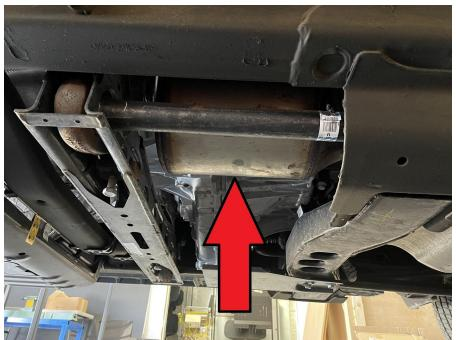
3.) There are two small holes located just behind the catalytic converter on the subframe near the steel joint toward the outside of the vehicle. Use your 25/64" drill bit to open the most rearward hole. See pictures.
