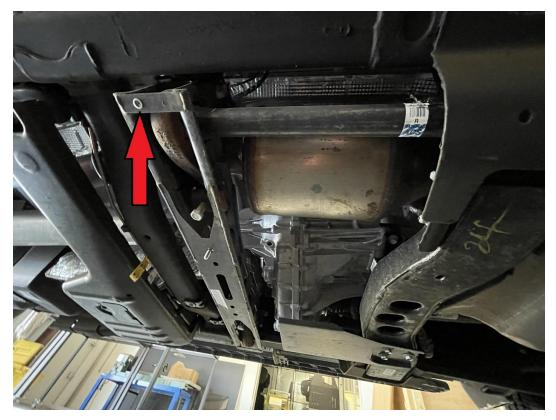
5.) Drop a 5/16"-18 x 2" bolt down the hole shown in the subframe. Feel free to use the washer supplied under the head. This bolt serves a temporary purpose for now.
