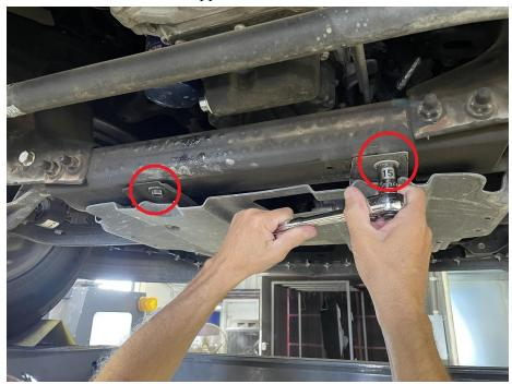
3.) Move to the rearward/mid subframe and identify the 4 holes/slots on the left and right.
