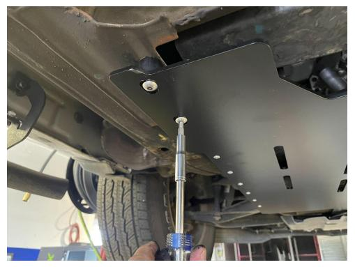
6.) Mark the rearward middle slot on the frame. It needs to be marked so you can know where to drill a hole and install a rivnut.
