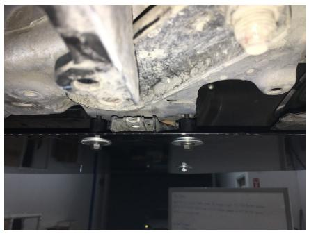
7. Go around and tighten all of the bolts/nuts on the underside of the splitter.
