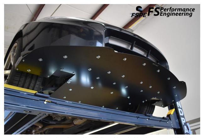
8.) Install your rods. Use the splitter rod installation guide to do this. There are pre-drilled holes in the splitter for this. This is where we installed our rods.
