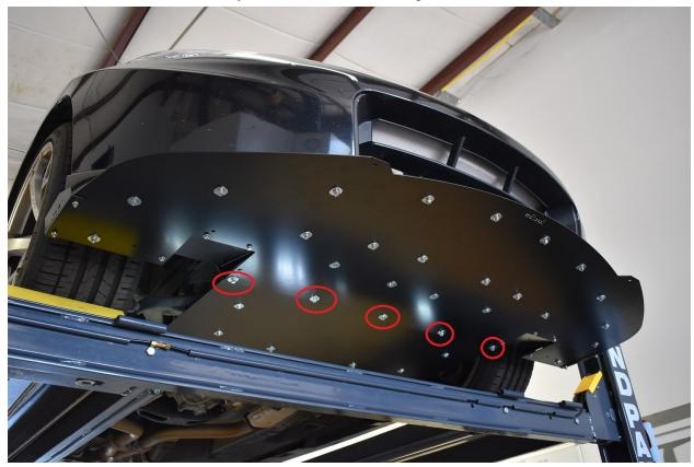
7.) The remaining holes in the under tray use various spacers and bolt lengths. All of them use 1" OD fender washers and ½" lock washers under the bolt heads.. Here is a top-down schematic of what goes where. Tighten them securely. Then tighten the ones from the previous step.
