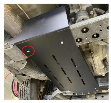
7.) The last mounting hole on the frame needs to be drilled out. Use a drill and 5/16" drill bit. Push the bit up through the guard, through the bottom hole crossmember, and into the interior of the crossmember you're drilling into. Drill through it.
