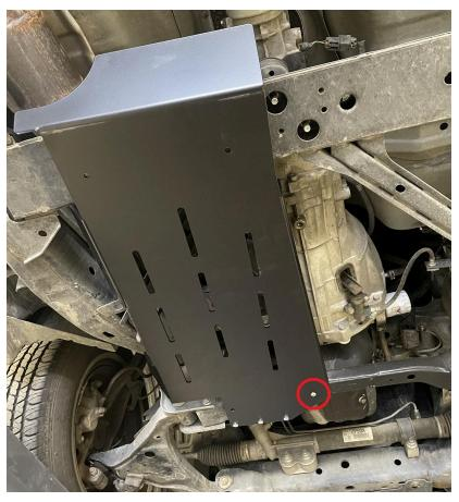
5.) Install a 5/16"- $18 \times 3$ " HEX bolt into the hole shown below. Push it through the frame and use a 5/16"x1.25" washer and 5/16"- $18 \times 18$  nyloc nut on top. Securely tighten.
