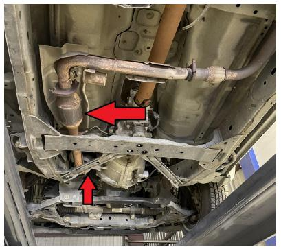
4.) Install your catalytic converter guard onto the vehicle using the M8-1.25 x 25mm security bolt. There are already threads in the vehicle. Use blue threadlocker on the threads. The security bit fits into a  $\frac{1}{4}$ " socket.
