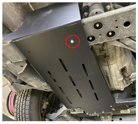
6.) Install a 5/16"- $18 \times 2$ " SECURITY bolt into the hole shown. Push it through the frame and use a 5/16"x1.25" washer and 5/16"- $18 \times 18$  nyloc nut on top. Securely tighten.
