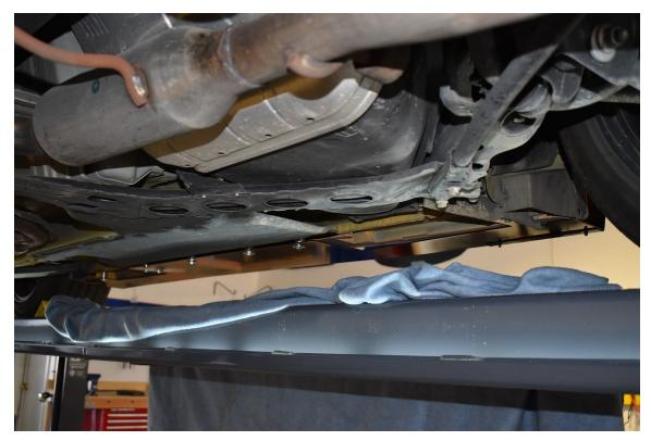
5. Using your 90 degree phillips head screwdriver, remove the phillips head screws found at the front rockerpanel - the rear two were already removed. If your car had mudguards you will have two at the front... if not you will only have one.
