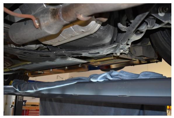
5. Using your 90 degree phillips head screwdriver, remove the phillips head screws found at the front and rear rockerpanel. If your car had mudguards you will have two at the front... if not you will only have one. Our pic shows two. You only have to remove the lower one at the rear. (SEE PICS)... FRONT:
