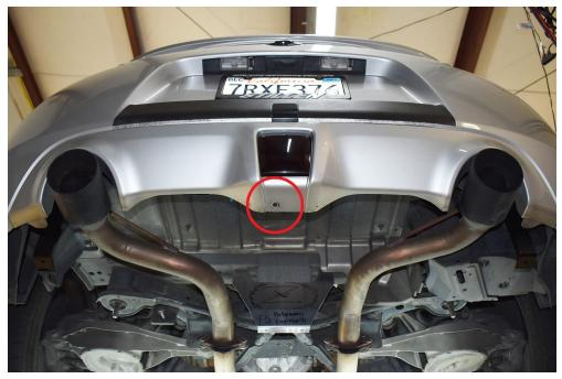
7. Install your diffuser onto the Z bracket, and the L brackets using the M6-1.0 x 20mm bolts pointing upward and nyloc nuts on top. Be sure to use the 1" OD fender washers on the bottom, and small washers on top. Then, use your M6-1.0 x 40mm bolt & and nyloc nut for the center hole all the way up through the bumper applying the washers as described before; in between the diffuser and bumper use the angled spacer. (pics below will show it all!)
