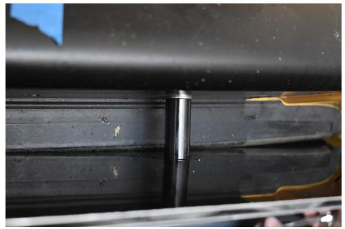
10.) Once the holes are drilled remove the three bolts mounted to the chassis into the M6 rivnuts, and install your 4 bolts at the front. If you have a 2nd layer then place it underneath. You'll be using four M6-1.0 x 65mm bolts with 1" OD washers on bottom, 45mm spacers between the splitter and bumper, and 1" OD washers on top with M6 nyloc nuts. Securely tighten.
