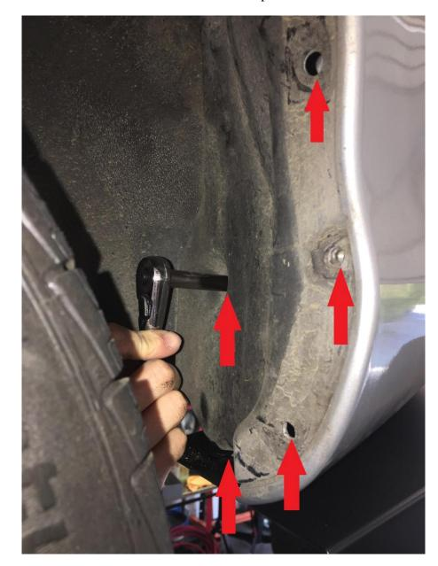
3. If mudguards are not installed, remove any screws or clips/fasteners to allow slight movement of the inner fender near the rear bumper. See illustration below.
