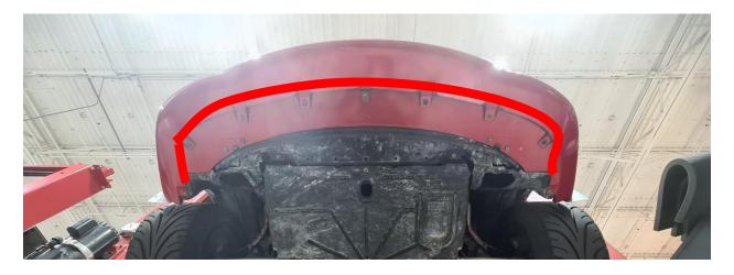
If you have a MAZDASPEED you have to remove the factory air dam before installing our Splitter Kit
