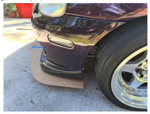
Now it's time to Install the splitter rods, these bolt to the bumper reinforcement which is located in the inlet area of the front bumper.
