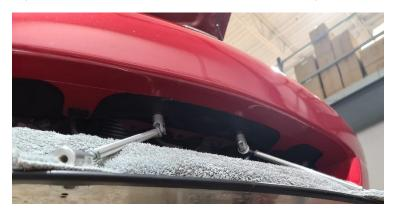
7. Now it's time to bolt your rods to the splitter and do final adjustments. For this you will use the 3/16" Allen.
