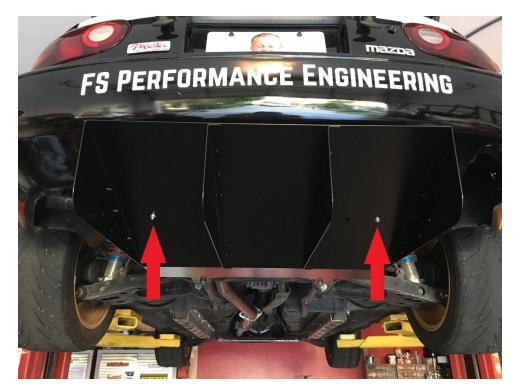
6. Install the remaining four M6-1.0  $\times$  20 mm hex flange bolts and nuts with the bolts facing toward the car (nuts on top). Hand tighten.
