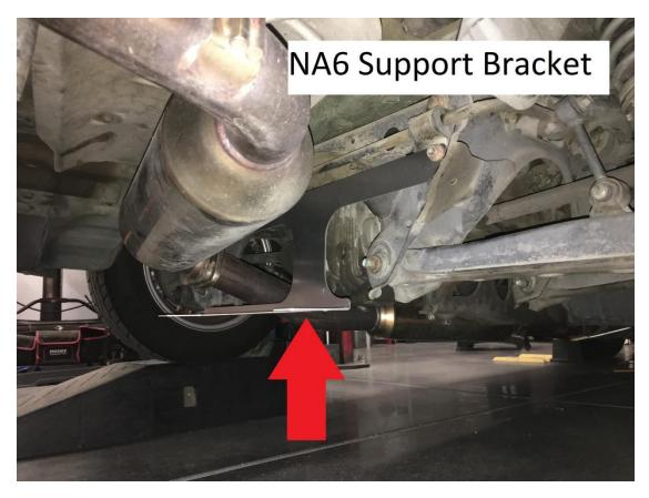
5. Drop two M6-1.0 x 20 mm hex flange bolts into the outer two holes of the rear bracket. Install the center diffuser with two M6-1.0 hex flange nuts and hand tighten.
