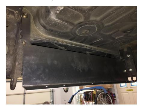
4. NA8/NB Miatas: Remove the two 17 or 19 mm bolts from the rear subframe.
