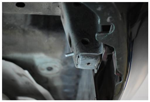
BLOCK THING WITH A M6 BOLT AND '4" SMALL WASHER BEING PUT THROUGH BIG HOLE INTO SMALL HOLE ON SIDE. We used the magnet here.
