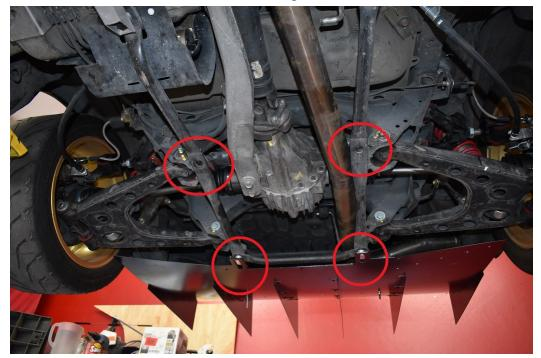
8. Panels 3 and 4 are going to be overlapped. **Panel 3 will be under panel 4**. Install panel 3 using two M6-1.0 x 20mm bolts and two fender washers at the front on the mounting rails. Overlap panels 3 and 4 and install them into the holes in the middle of the bracing from step (7.) using two M12-1.5 x 60mm bolts + two M12 fender washers + two 30mm spacers between the panels and subframe bracing. See several pictures below. Finger tighten everything.
