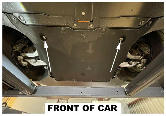
2.) Next, on the bumper's undertray remove the 10 clips that help hold it in place using a flat head screwdriver or clip remover.
