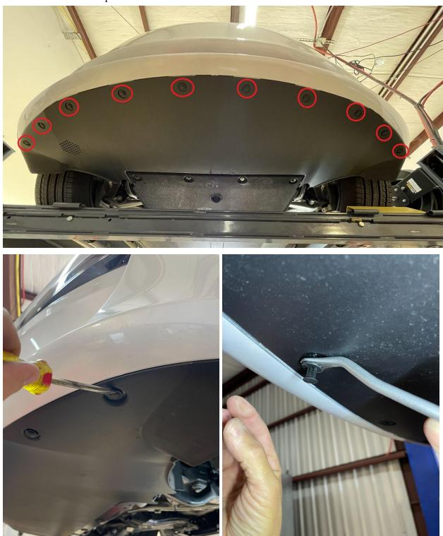
3.) There are also 2 clips on each side (4 total) on the interior of the fender well that need to be removed. Don't remove the third clip that is closest to the outside of the car.
