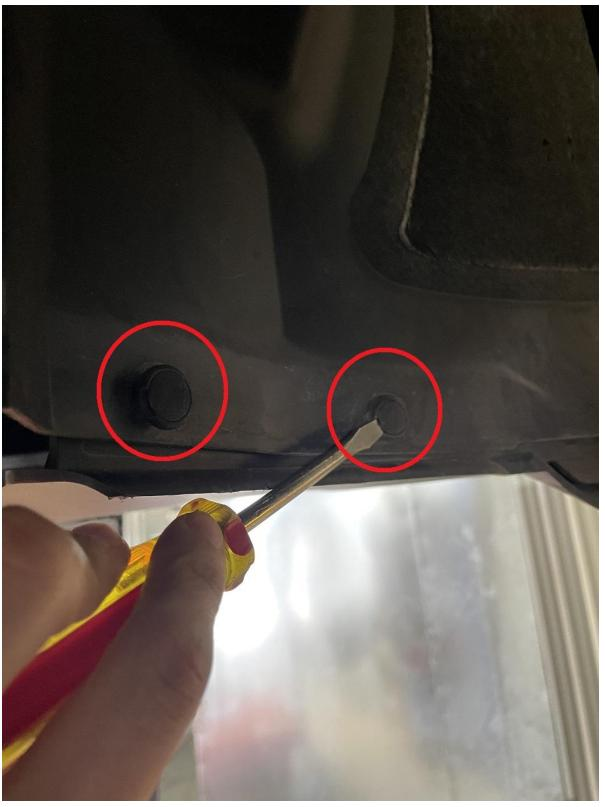
4.) Now you can install your splitter into the 10 holes along the bumper. All holes will utilize the same bolt length. However, some of them use spacers between the splitter and car as shown:
