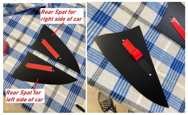
4.) Push the car's bolts upward through the spats and line them up with the holes in the car where the bolts were removed. Securely tighten with your 10mm wrench. The 3M tape will make contact with the underside of the bumper.
