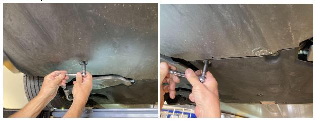
5.) Now you must identify where the fins will mount. The most inner fin is the longest. All tabs on the fins fold toward the inside of the car. Place blue masking tape at the location shown (we started with the left fins).
