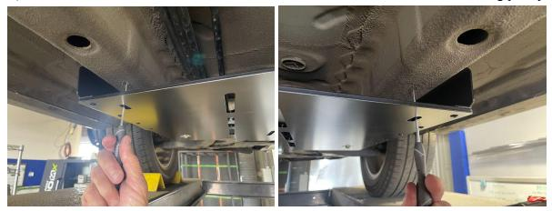
6.) Remove the guard now, and drill out the marked holes and install 5/16 rivnuts.
