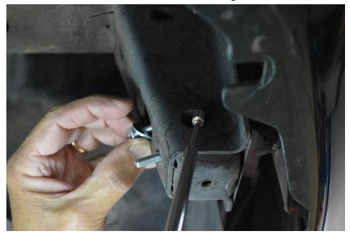
WHAT IT LOOKS LIKE WHEN BRACKET IS INSTALLED... <u>except your tab on the</u> <u>bottom will be folded the opposite way!!!</u> Use the WIZNUTS here and threadlocker if you want. Do both sides and tighten securely.
