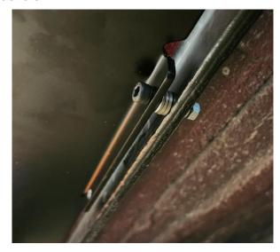
As shown in the picture above you will use the washers as spacers. Depending on your car in can be 2 or 3 per bolt. **NOTE: The picture above shows a prototype Allen bolt, your kit will have an 8mm head M5 bolt instead for this application.**
