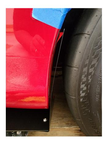
This next part can be done two different ways, either remove the tape completely and then bolt the wicker to the sideskirt or lift the tape a little bit and bolt the wicker to the sideskirt.
