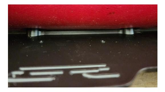
A Delrin Angled Spacer (shown in picture above) ensures that the sideskirts sit at the perfect angle and the underskirt billet washer (shown in the next picture) provides the new, longer stainless-steel bolt a flat surface to rest on, since our sideskirts are parallel to the ground and the bolts go in at an angle.
