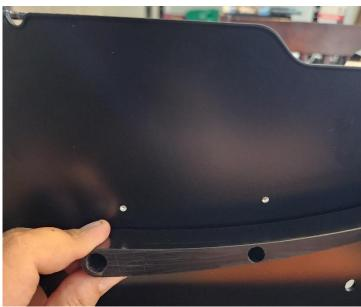
The underskirt airfoils go underneath the skirt, they have a specific direction, and they are also specific to one side. The airfoil pictured above goes on the left (driver) side. No matter the side they are always pointing out.
