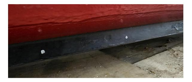
Before marking your holes make sure that the sideskirt is straight. Drilling the holes too high or low will create a bump or dip on the straightness of the sideskirt. So, take your time, take a good look and use a level if necessary.
