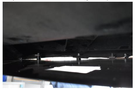
8.) The rear 4 holes double as holding up the splitter and rear tray. Use M6-1.0 x 40mm bolts to secure it. Under the heads of the bolts use  $\frac{1}{4}$ " lock washers and 1" washers. No spacers used here, just make sure you tighten well.
