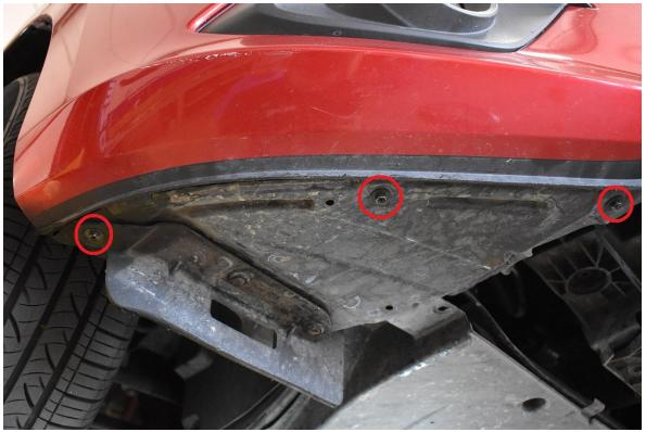
4.) Remove the "flaps" that hang down on each side using your flat head screwdriver. There should be 3 pop clips.
