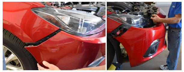
To fully separate the bumper disconnect the fog light wires on both sides. Set the bumper aside.
