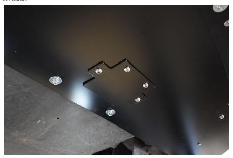
10.) Install the winglets. Use the counter sunk hardware. USE OIL ON THE THREADS WHEN TIGHTENING - don't over tighten.
