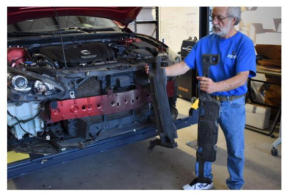
Now you can install the splitter rod brackets. They are located 6  $\frac{5}{8}$ " from the center of the crash bar. The top of the chassis bracket meets the top of the crash bar. Use a level to vertically align the brackets. Mark the holes and drill them out with a  $\frac{1}{4}$ " industrial rated drill bit. They are installed with M6-1.0 x 20mm bolts,  $\frac{1}{4}$ " small washers, and nyloc nuts.
