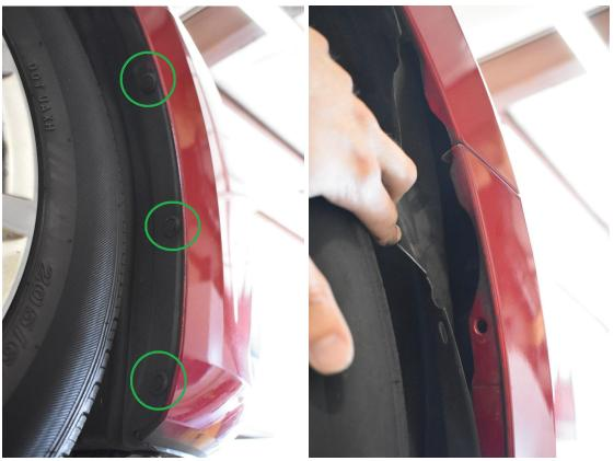
Remove the bolt on each side of the upper fender wells (8mm head).
