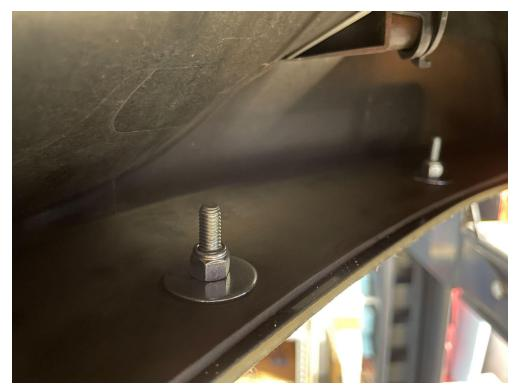
5.) Before buttoning things up, you need to identify where splitter bolts are interfering with your skid plate. We found that the center FIVE bolts will interfere. You need to "notch" out pieces in the skid plate for them. We used diagonal cutters to create v-shaped notches so the bolts don't run into the skid plate.
