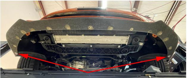
3.) Next, squeeze the front of the splitter and bumper together. Align the two together so the interior contours match. While holding it, drill a ¼" hole up through the bumper. Have a friend help if necessary. Then install a bolt and nut with washers on top and bottom. (see pics)
