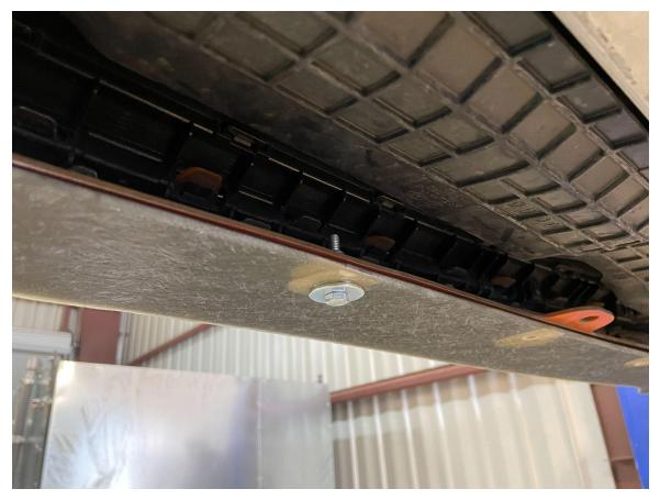
4.) Now you can drill into the bumper through the remaining holes in the splitter, and then install the remainder of the splitter with your bolts, nuts, and washers. Assure you are putting washers on top and bottom and secure the splitter tightly.
